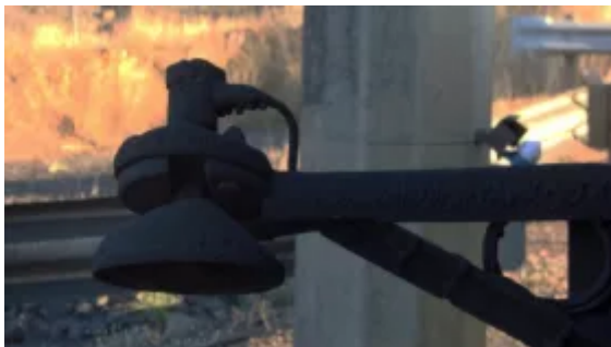
Fig. 4: Radar sensor with parabolic antenna for monitoring a coal unloading station.
