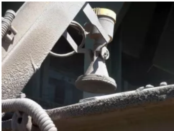
Fig. 7: Measurement of crusher filling level in a copper mine by radar.
