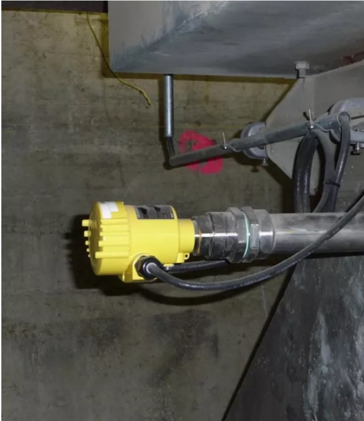
Fig. 2: Microwave barrier with tube extension for temperature decoupling in a clinker
