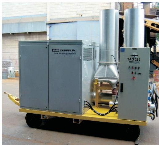
AGU - Air generation unit
