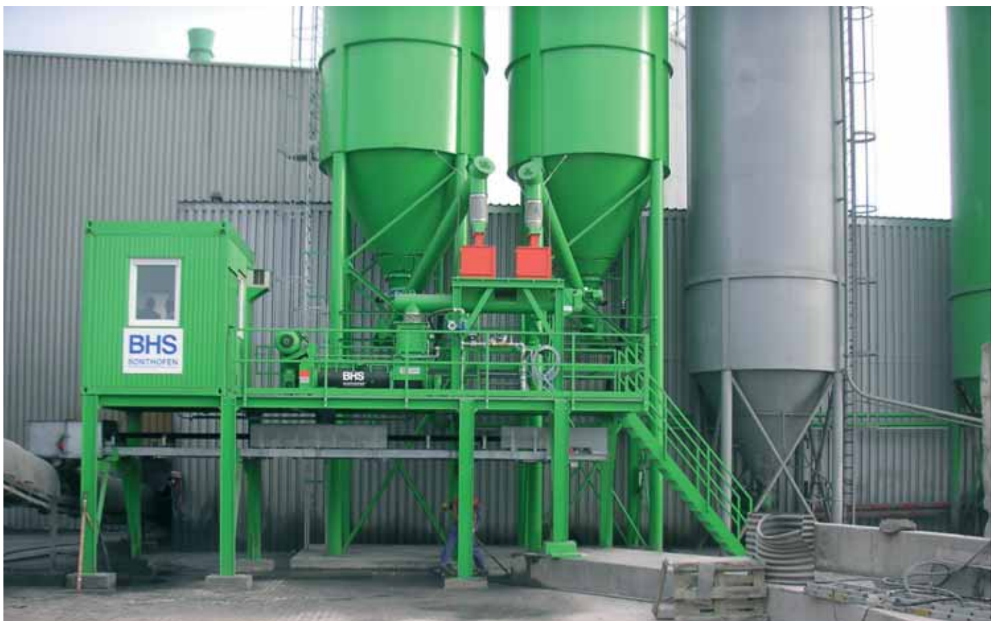
Complete BHS Mixing Plant for continuous moistening of fine materials, installed at one of our customers in Southern Germany.
