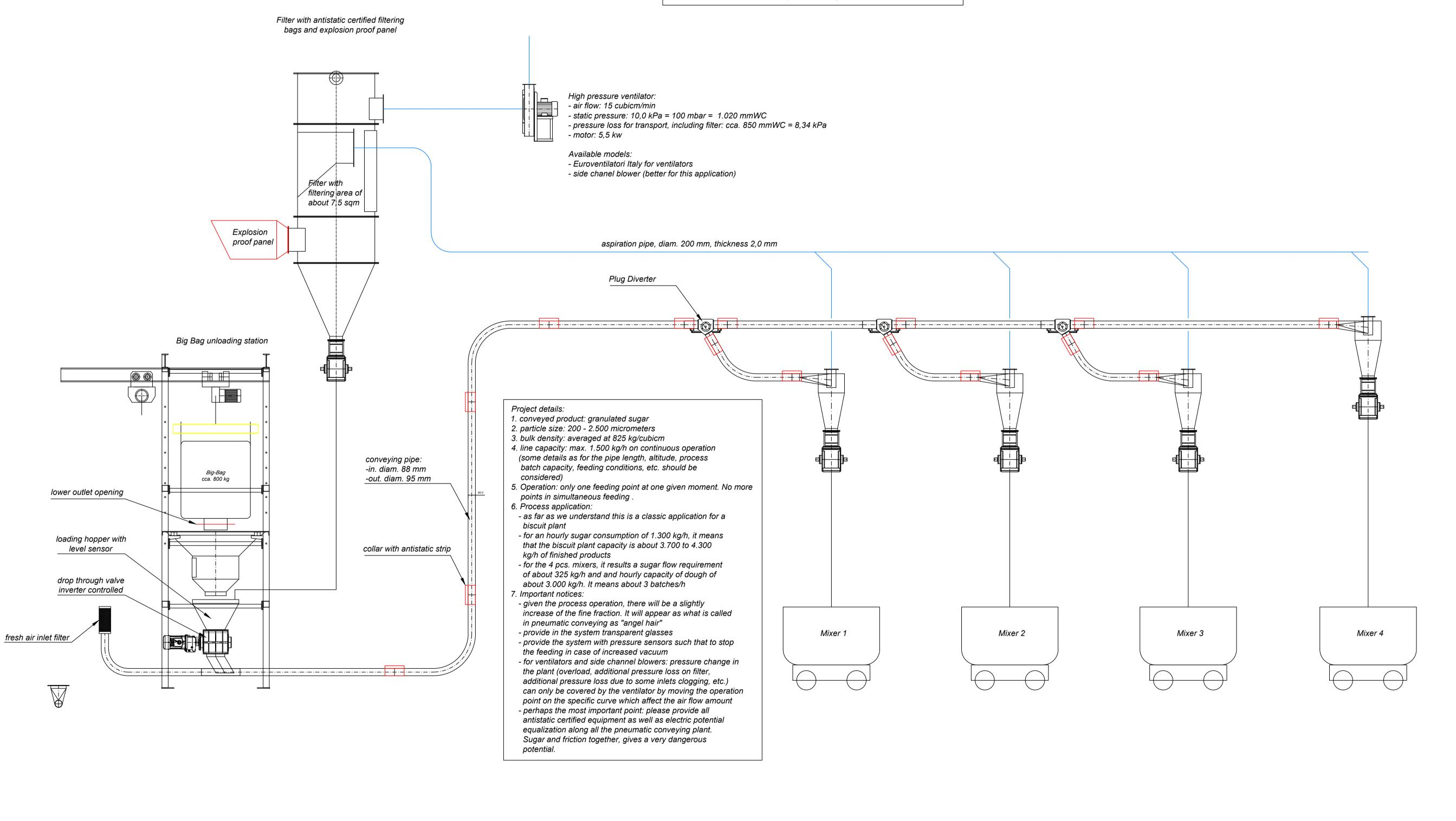
Project: Pneumatic Conveying plant for Sugar - preliminary lay-out, cap. 1.500 kg/h
