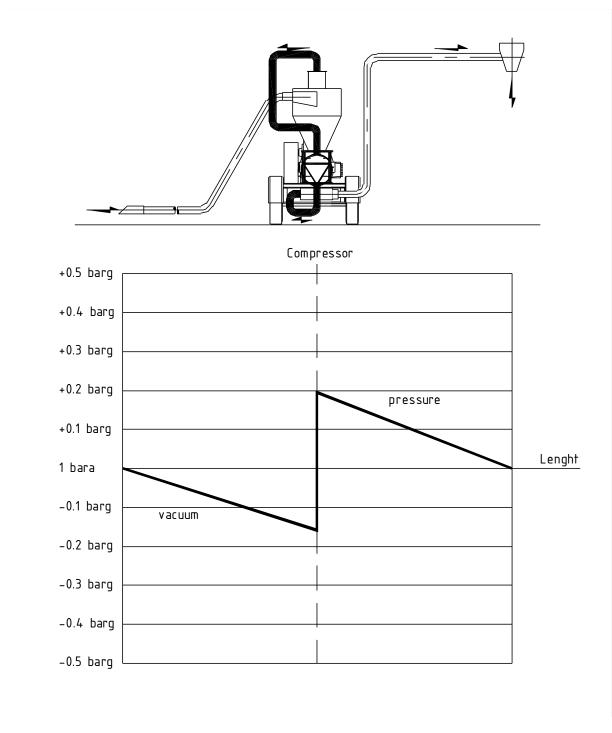
Drawing 1: Continuous mobile vacuum-pressure unit, using one blower
