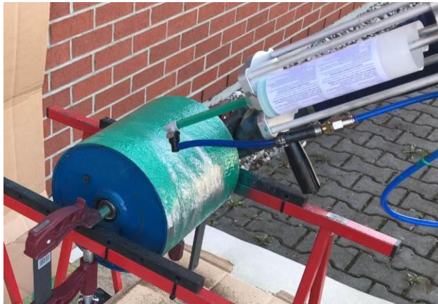
Apply and spread Multi-EP with a spray gun or a brush or a spatula
