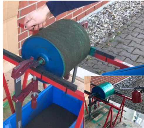
Apply blasting grit manually or with a gritblasting gun
