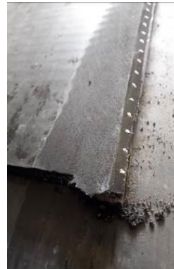
Steel cord belt edge repair
