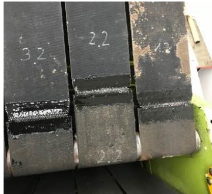
Overcoated belt fasteners
