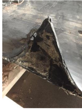
Splice repair on the belt edge
