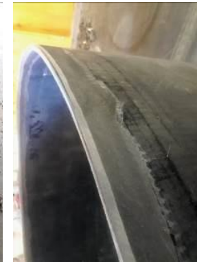
Steel cord belt edge repair
