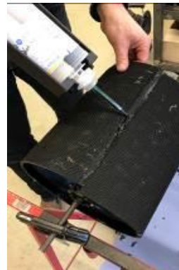
Pulley lagging joint filling
