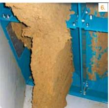
6. Paste-like Filter Cakes from Bunker with a Capacity of 300 m<sup>3</sup>
