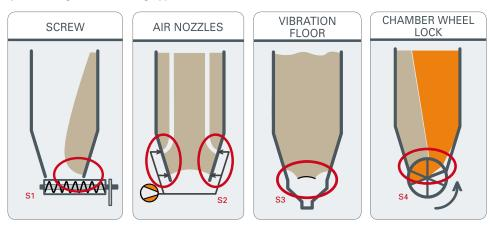
S1 Uneven discharge of screw conveyors forms dead zones in the silo.
