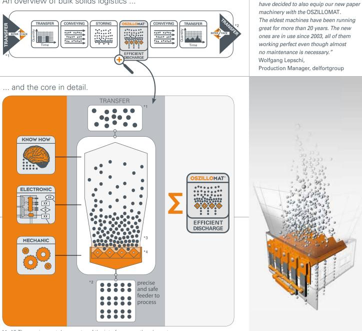
\*1, \*2 The requirements/ parameter of the interfaces or rather downstream processes are considered in \*3 design/dimensioning of the silo geometry and \*4 the oscillating beam floor.
