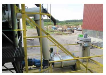
Installation with TP Screw Feeder, DUSTFIX® and WAMFLO® Dust Collector
