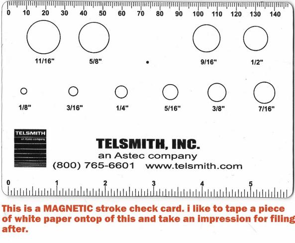
Note: quite often we just use this magnetic card to see what stoke shows up by identifying which circle size shows a nice clean DOT in the middle as the stroke the machine is operating at. FOR horizontal you will get a line at an angle which actually indicates the TIMING ANGLE of the gears.
