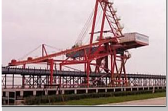
5000t/h Ship Loader for coal
