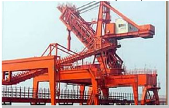
4500t/h Ship Loader for Iron ore
