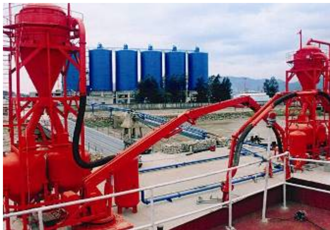
300t/h Pneumatic Ship Unloader
