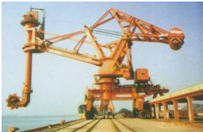
1600t/h bucket wheel ship unloader for iron ore
