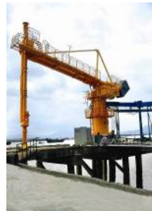
350t/h Screw Ship Unloader
