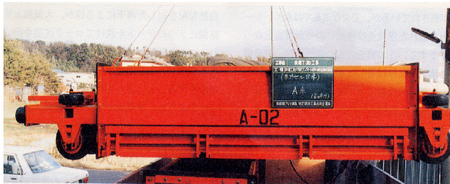
Figure 4 A capsule of the rectangular type used in the construction of the Akima tunnel
