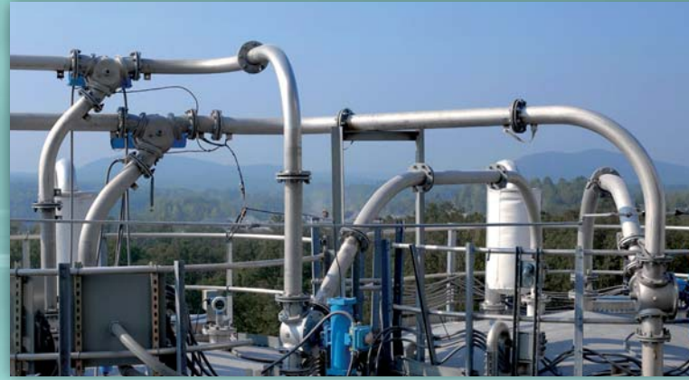
Dilute Phase Conveying system with long radius elbows
