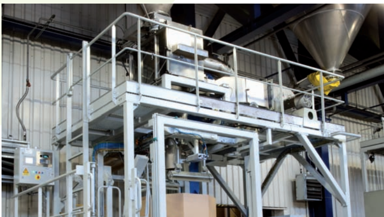
Delaere big bag loading station with integrated Pelletron DeDuster ®
