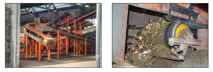
NUOVA GEOVIS SpA is responsible for the recycling services in the Italian area of Emilia. Rulmeca is cooperating to replace all exposed drives with Motorized Pulleys, due to improved efficiency, minimal maintenance and the compact design our Motorized Pulley can offer.
