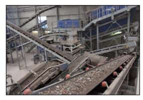
The environment is dusty, abrasive and corrosive. The Rulmeca products supplied are Motorized pulleys 220M, 320M, 400H as well as idlers.
