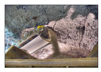
**ITALY**Rulmeca PSV rollers D.89-108-133/20 and Motorized Pulleys 400H-M 11kW-7,5kW working at Unicalce Group, a Lime Stone Mining.
