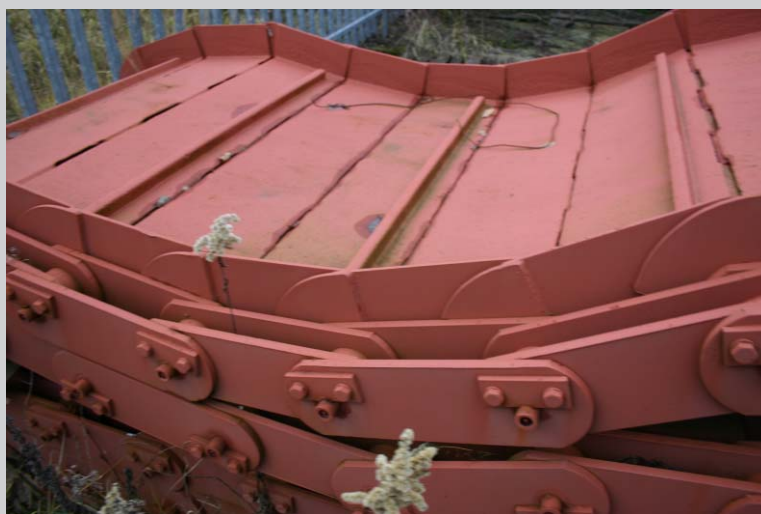
Fig. 2: Apron feeder of the hammer crusher
