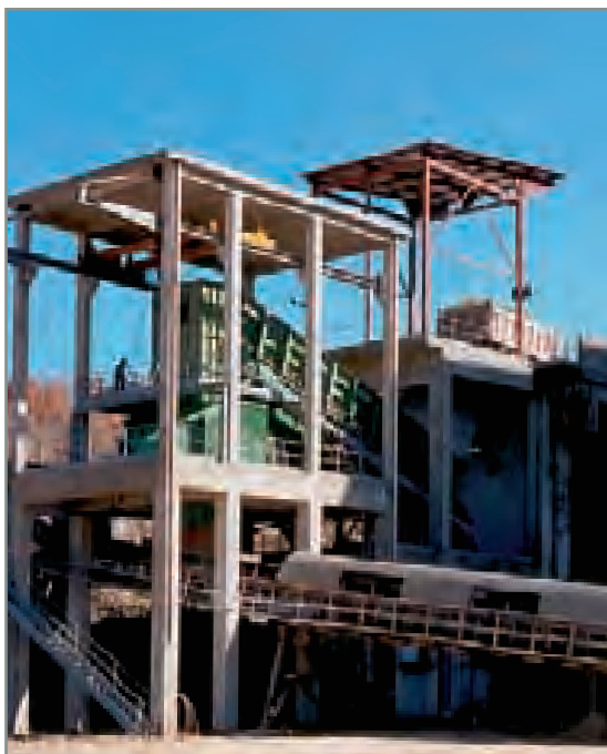
Different types of primary and secondary crushing groups, stationary or semi-mobile, for limestone as well as moist and sticky materials.
