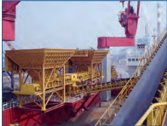
Grab cranes and selfunloading bulk carriers (offshore application). Capacity up to 5000 m 3 / hour
