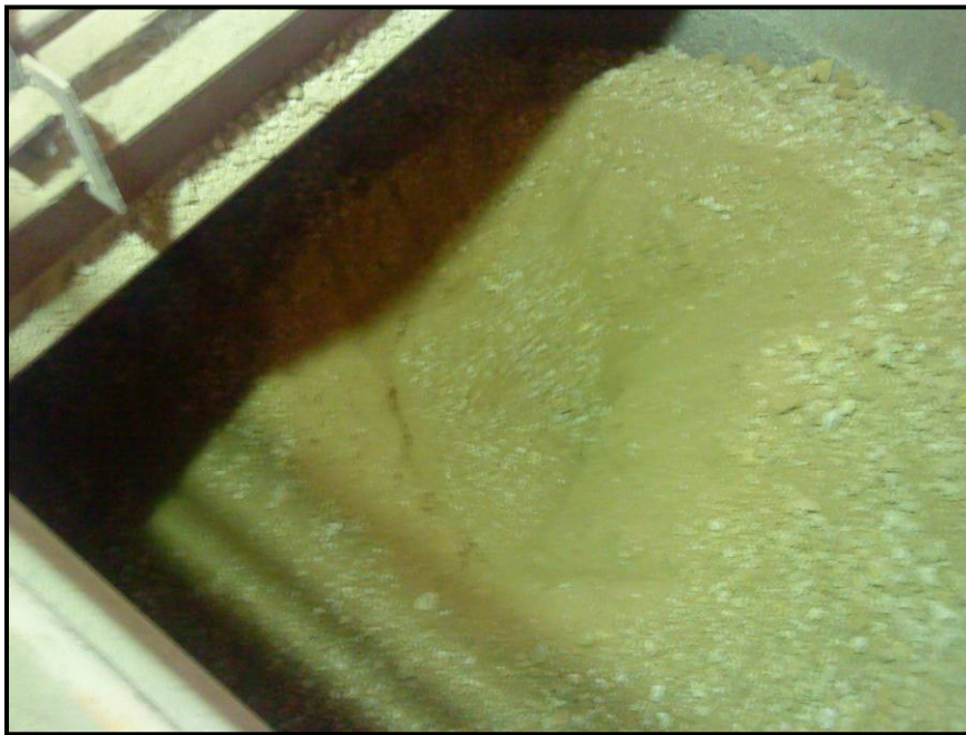
Fine particles segregation in the back end of the bin
