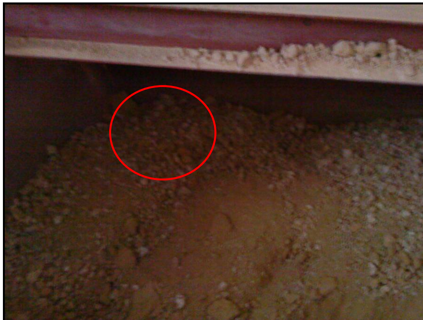
Coarse particles segregation in the front end of the bin
