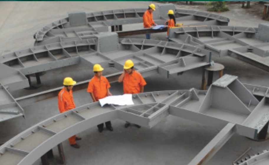
Dumper fabrication and quality control
