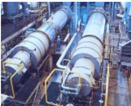
Twin rotary system for reclaiming aluminum scrap
