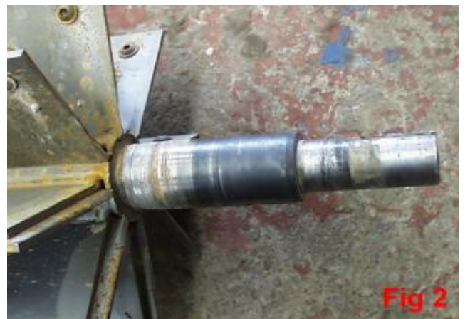
Fig 2 HARDENED STEEL SHAFT LINER
