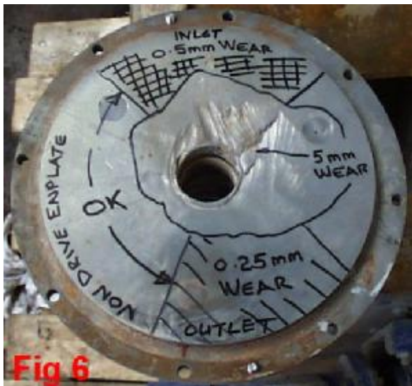
Fig 6 NI-HARD LINED NON-DRIVE ENDPLATE
