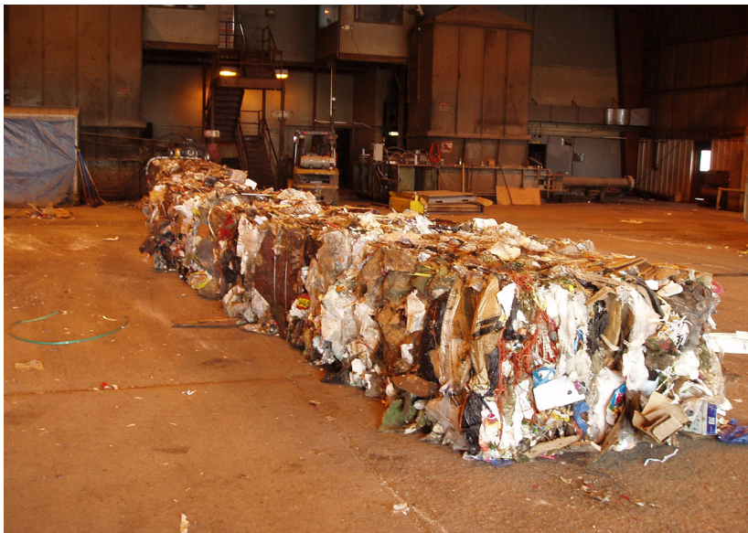
Baler in Operation (MSW 2200 # Bales)
