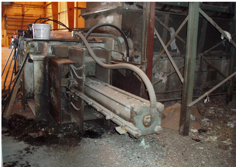
9 inch Ejection Cylinder / 95 Tons Force
