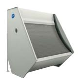
Sta-Sieve® Stationary Screening Devices. Provides quick and efficient separation of solids from liquid. Ideally suited for processors that use large quantities of water. Advantages of this low-cost unit include high flow rate, long screen life and no moving parts. Can be operated independently or as a system component in conjunction with Sweco Separators or Centrifugal Screen Concentrators.
