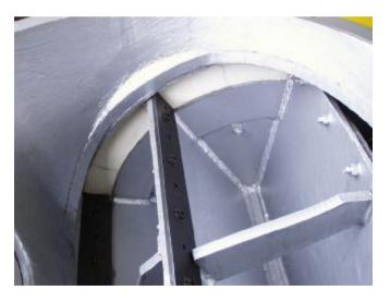
This is a rotary valve with a 670 mm diameter x 631 mm long bore, used for handling grain.
