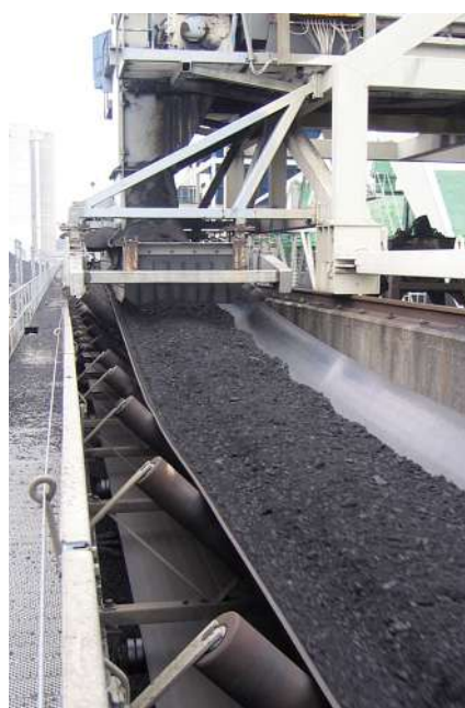
Fig. 3: Wear especially occurs at the loading point where the belt is exposed to impact.
