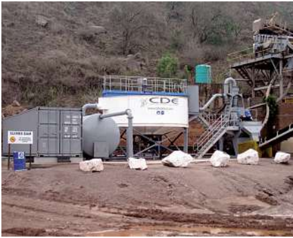
The Evowash system reduce the need to purchase natural fine sand from external suppliers.
