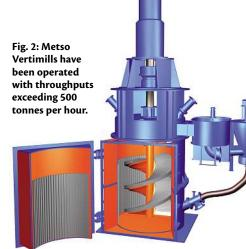
always significantly less than a traditional horizontal ball mill solution. The advantages of vertical stirred mills include:
