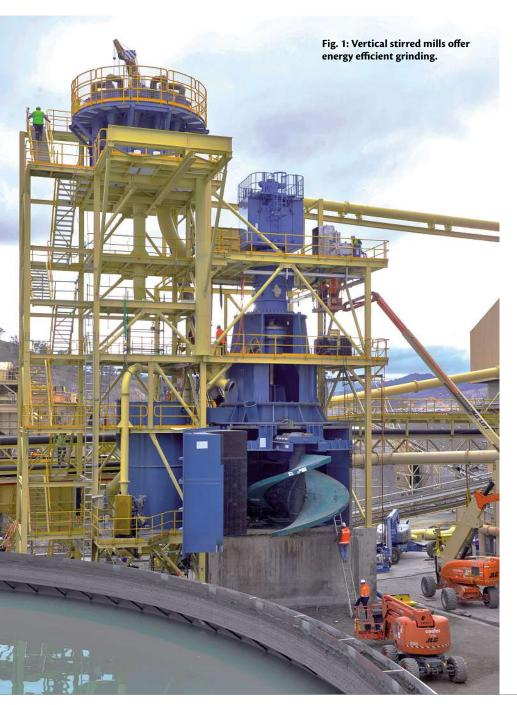
ertical stirred media mills are recognized as energy-efficient grinding machines, but reduced media consumption, lower installation costs, minimal maintenance, and minimal liner wear make the Metso Vertimill solution the lowest total cost of ownership in many applications, substantially improving the profitability of copper concentrators.
