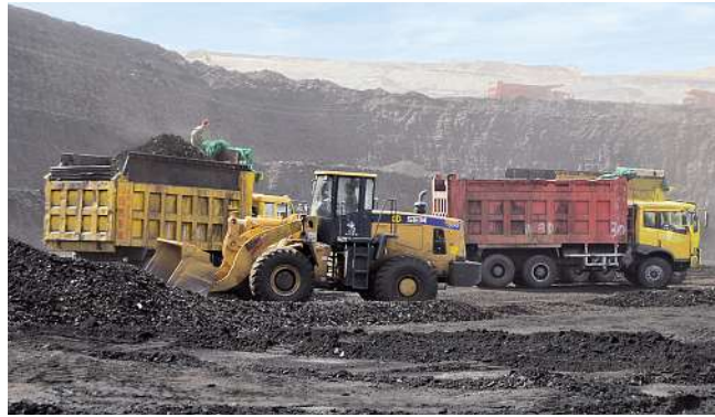
Fig. 2: Surface mining produces particle sizes smaller than 100 mm, trucks can thus accept more material per truck load.
