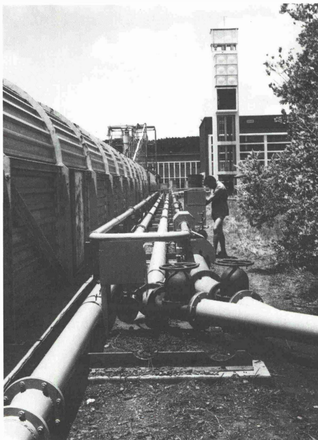
Fig. 2: The 100, 200 and 250 mm diameter slurry test loops
