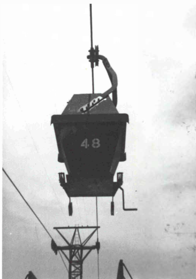
Fig. 5: Totally enclosed buckets for very fine material prevent dust being ejected on the line
