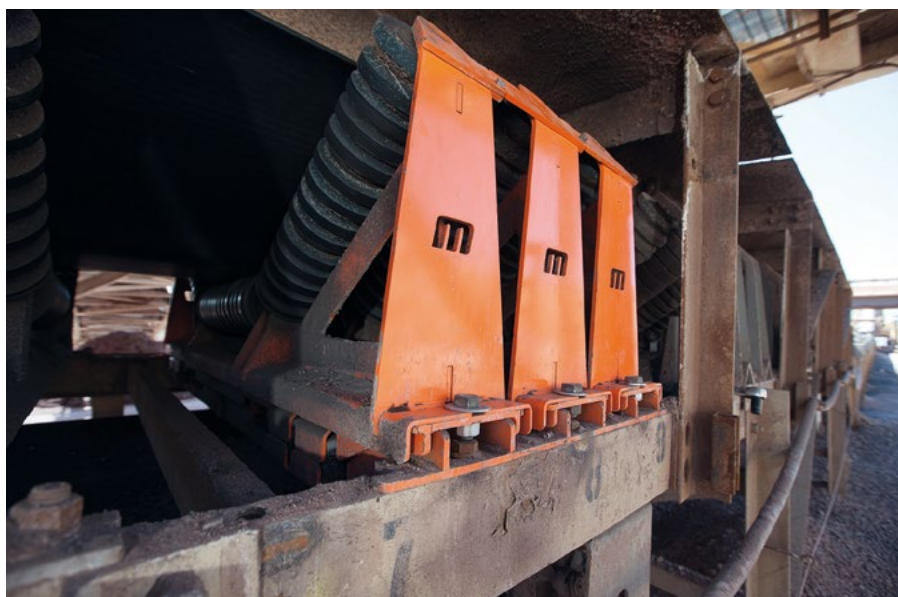
The new EVO High Speed Roller Cradle employs multiple heavy-duty impact rollers spaced close together in a track-mounted configuration.
