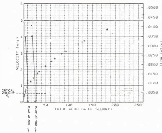
Fig. 6: System curves. These are derived from the friction loss curves, the slurry SG, the pipeline length and the static head applicable. Because static head is in metres of slurry head, the system curves are plotted in the same terms. Manufacturers' published pump curves can be plotted directly on to this system curve.
