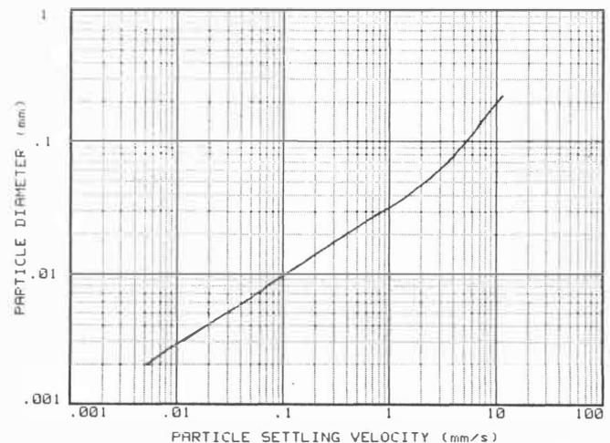
Fig. 2: Particle settling velocities in clear water (from laboratory measurements)
