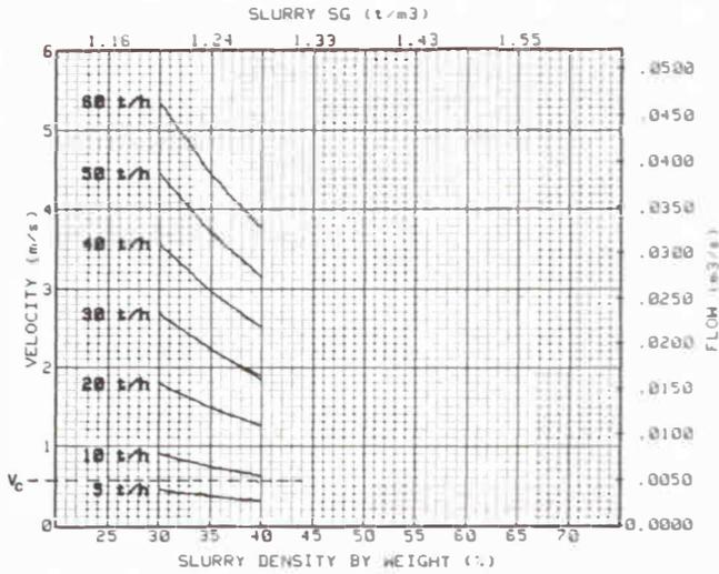
Fig. 4: Slurry throughput curves — this is a direct function of pipe size, slurry concentration and operating velocity. Critical velocity results can be superimposed on to this graph manually.
