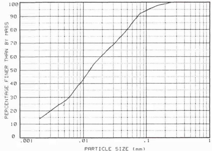
Fig. 1: Particle size distribution (plotted from data)
