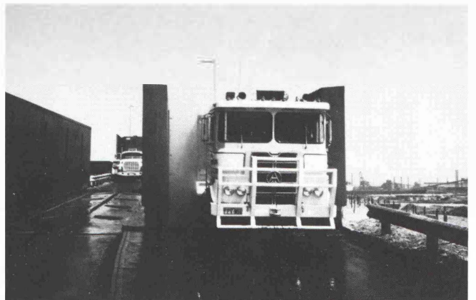
Fig. 5: After dumping, trucks are washed to prevent spilling dust on public roads. Extensive landscaping of 10,000 trees and 60,000 shrubs provides visual and noise shield.
