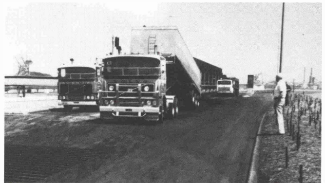
Fig. 4: Different grades of coal can be dumped by 9 trucks at the same time. Trucks are controlled by traffic lights mounted on the wind screen.
