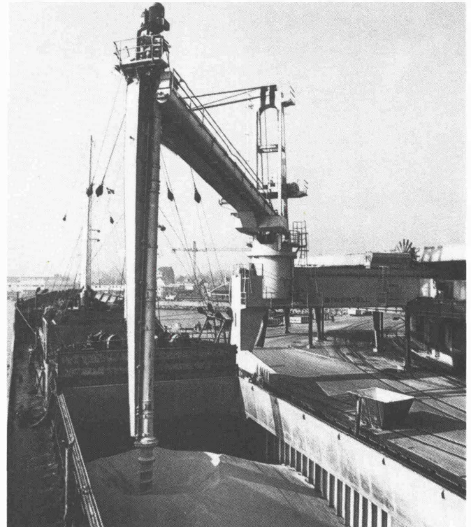
Fig. 9: Screw-type continuous shipunloader by Siwertell
