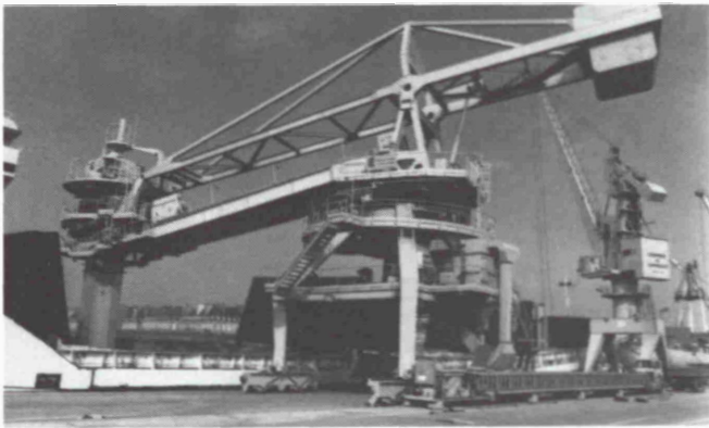
Fig. 5: Bucket elevator continuous unloader by Delattre-Levivier. This machine has a capacity of 1,000 tons per hour on phosphate
