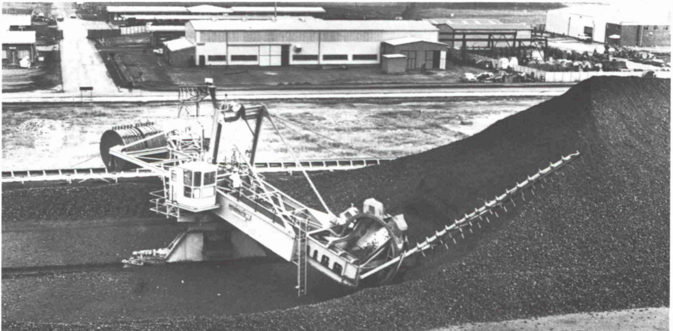
Fig. 13: The half-bridge boom-type bucketwheel reclaimer at Kleinkopje can equally well reclaim in both directions by simply slewing the boom around
