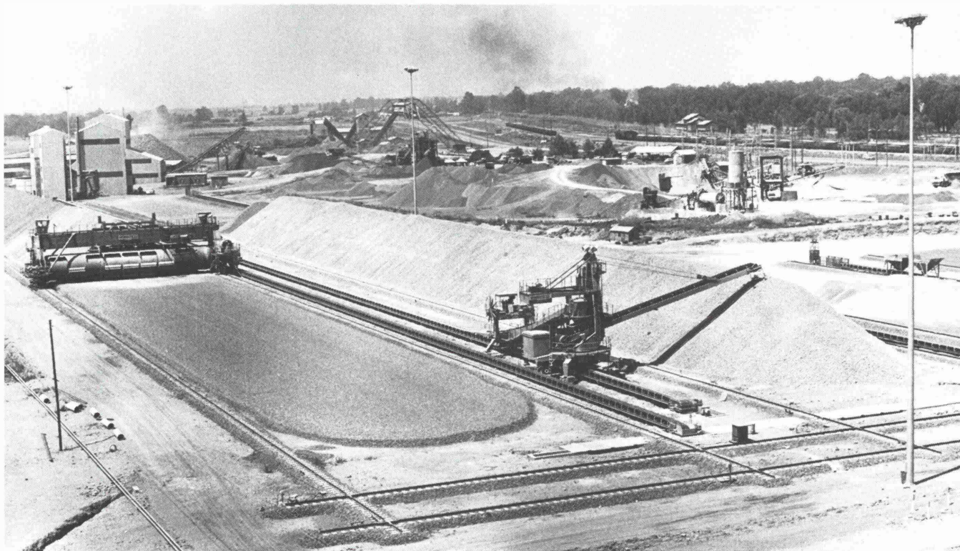
Fig. 4: Iscor's homogenizing plant at Glen Douglas for dolomite. The drum reclaimer is equipped with swivel bogies to transfer over the cross travel tracks in the foreground
