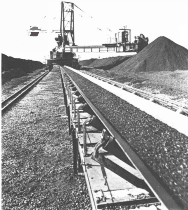
Fig. 6: The combined stacker/bucketwheel reclaimer at Vanderbijlpark homogenizes partially by a combination of windrow stacking and sickle-cut reclaiming
