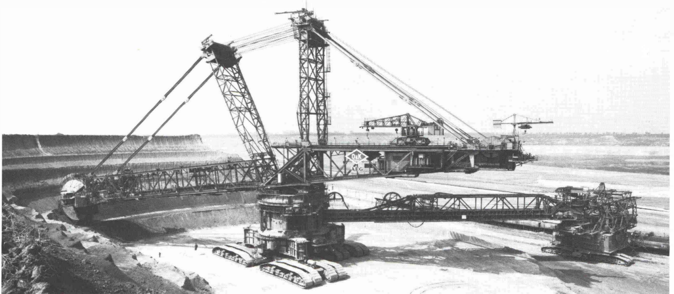
Fig. 4: The first "Giant Bucket Wheel Excavator" SchRs \frac{3600}{5} \times 48 with a daily output of 100,000 \text{bm}^3 ; put into operation in 1955.
