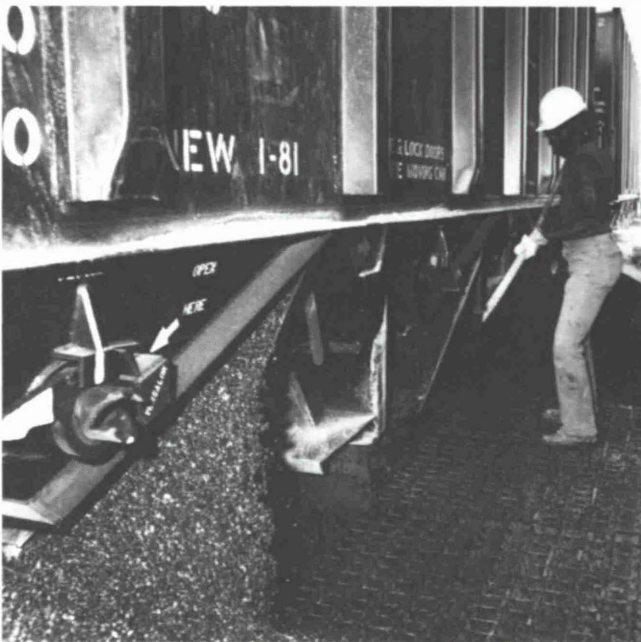
Fig. 5: At the South Pierce Chemical Works, one man can unload a car from either side. Each doorset is locked and unlocked with the yellow handle. The doors are then opened with a simple turn of a steel bar inserted in the locking hub.
