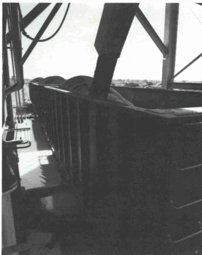
Fig. 1: Wet rock is loaded into Rapid Discharge ® cars at the Ft. Green washer
