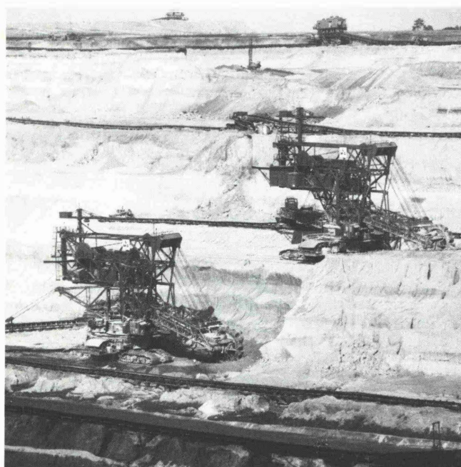
Fig. 18: Bucket wheel excavator in the brown coal area Neyveli/India
