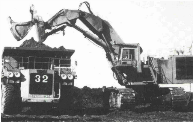
Fig. 5: Demag H 241 shovel loading oil sand onto trucks
