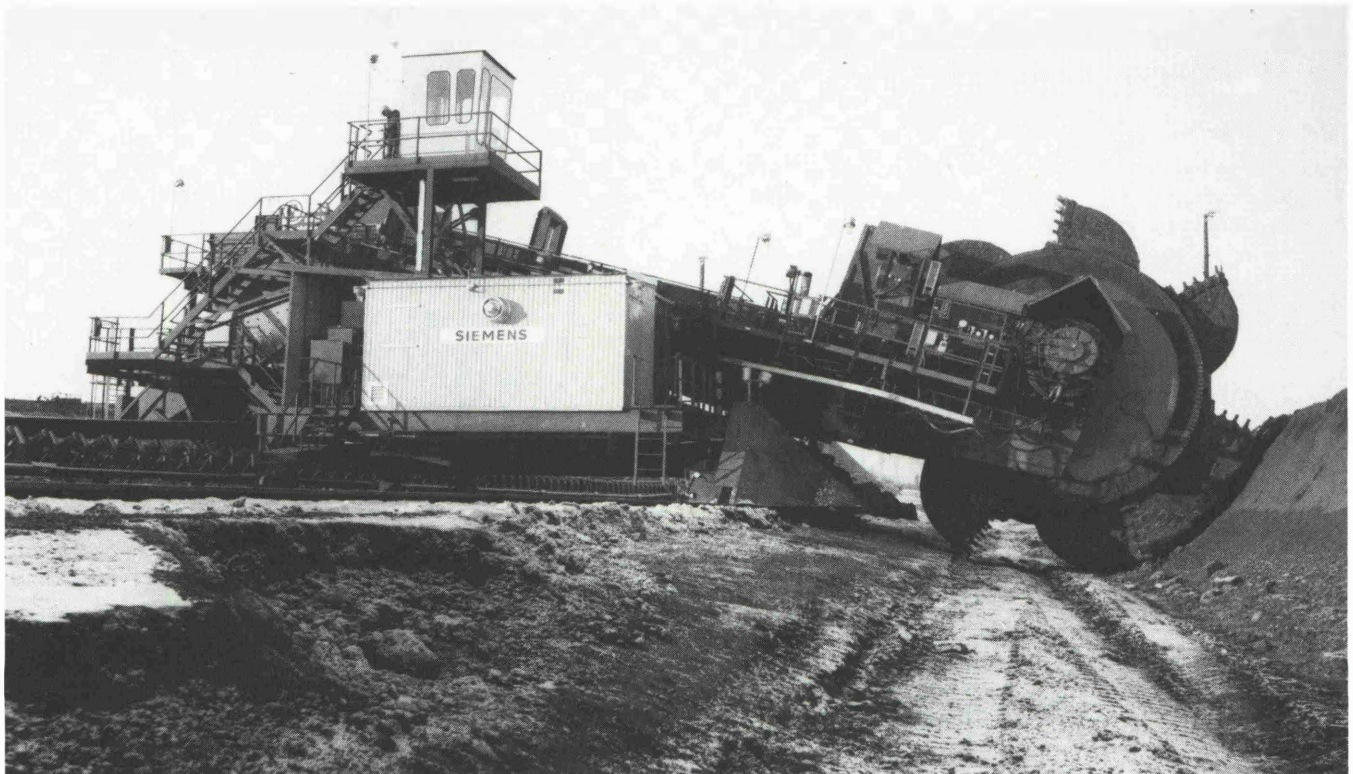
Fig. 6: Demag Lauchhammer trench reclaimer
