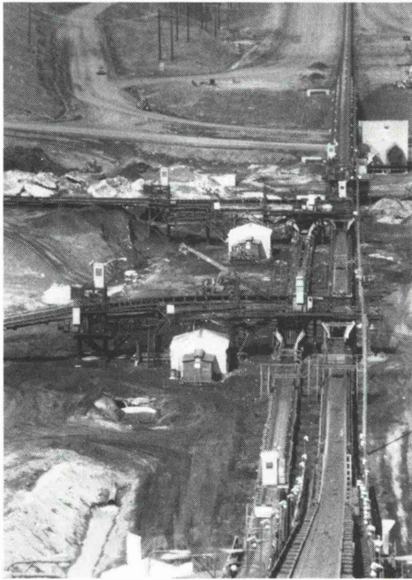
Fig. 1: Suncor conveyor system leading to extraction plant
