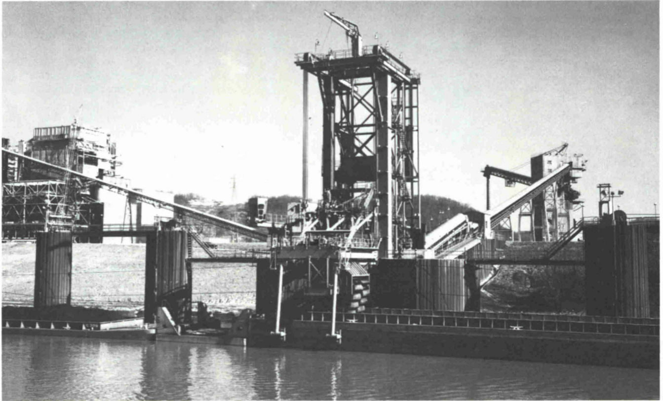
Fig. 16: This Twin Ladder 3,600 t/h continuous barge unloader can operate with a river elevation variation of 30 ft. Fast barge changing is accomplished with a patented "Shuttle Barge" haulage system.
