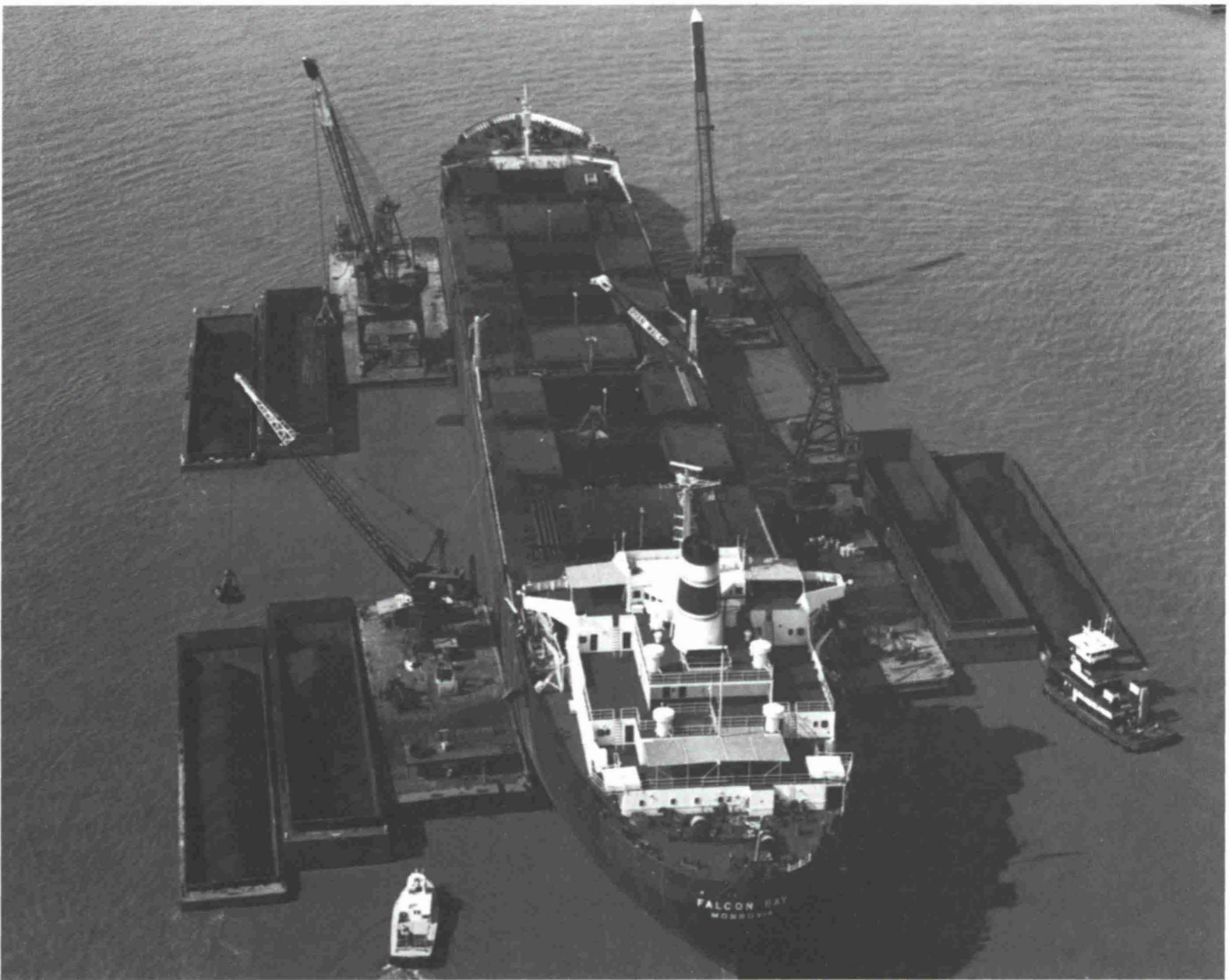
Fig. 19: Mid-stream coal transfer system (Courtesy Ryan-Walsh Stevedoring Co.)
