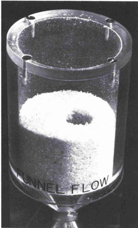
Fig. 1: Funnel flow Some material is stationary while the rest is moving
