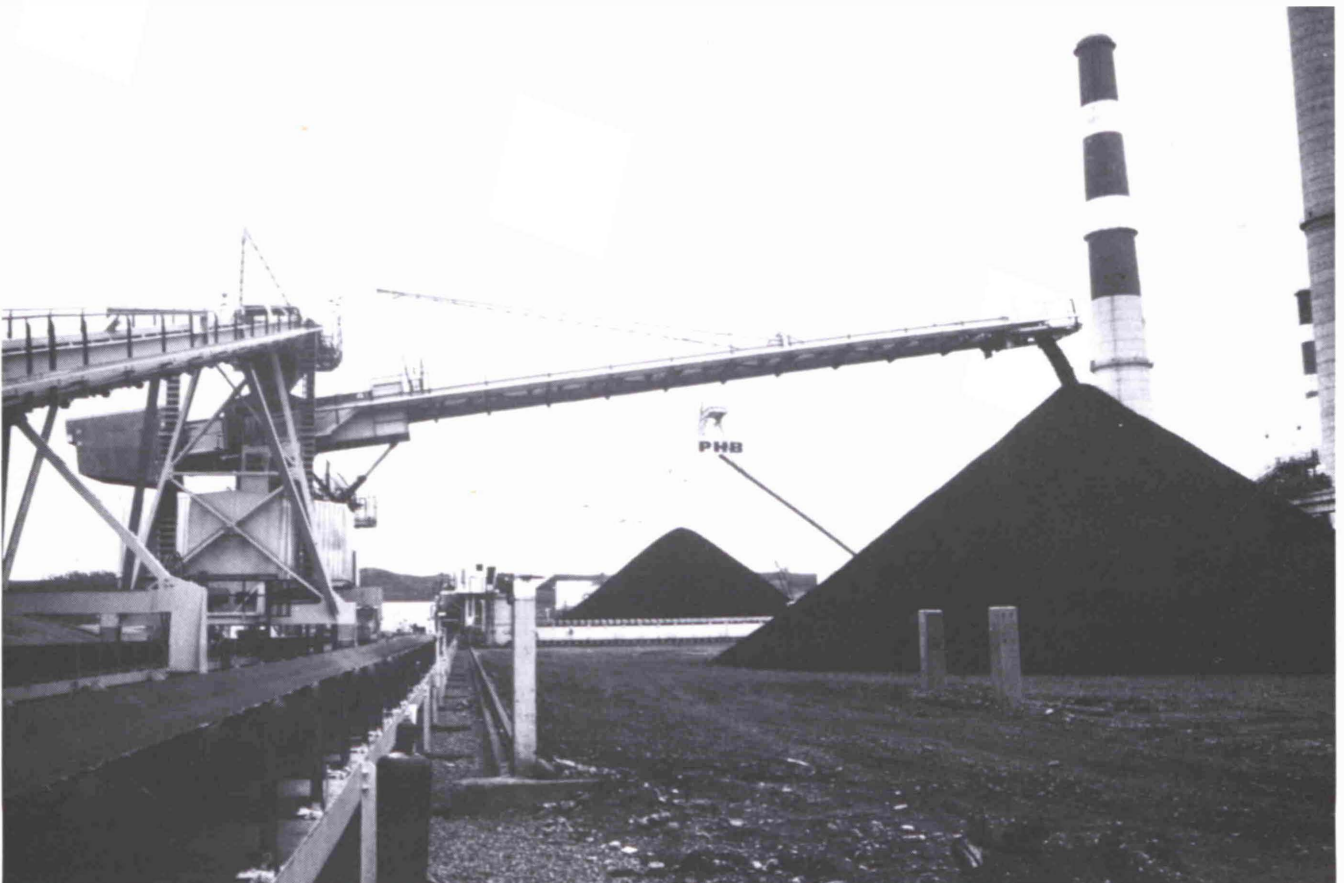
Fig. 4: Stacker und portal scraper reclaimer at Battle River power plant, Alberta, Canada
