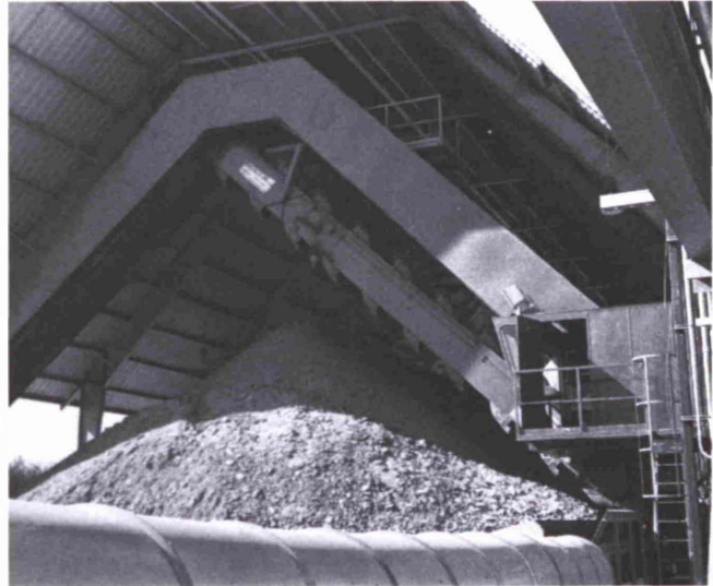
Fig. 8: Bucket boom portal reclaimer BEL P 100/14
