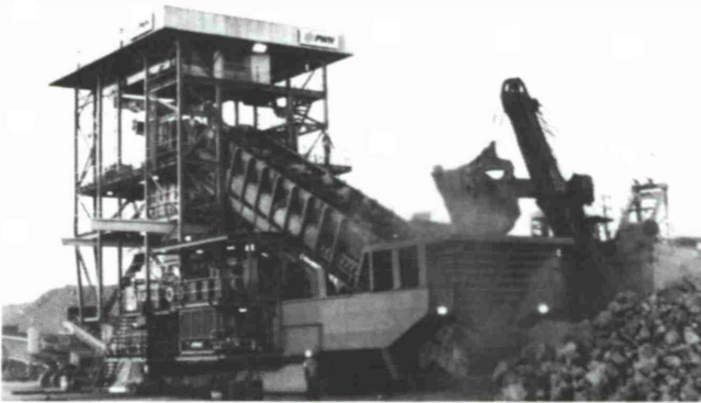
Fig. 7: Mobile crusher and shovel working as a unit (see Fig. 1)
