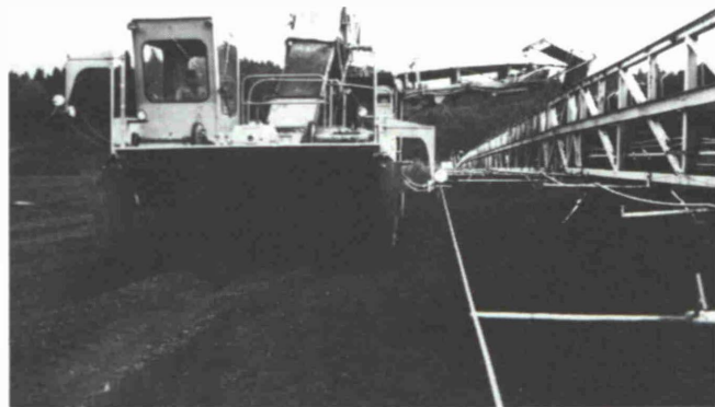
Fig. 6: Rotary drum reclaimer automatically following the guideline. The operator monitors the operation
