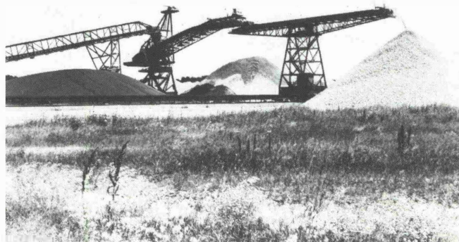
Fig. 5: Patented Soros slave stacking system builds third row of stockpiles, saving the capital cost of an additional 10,000 t/h yard conveyor, stacker and runway
