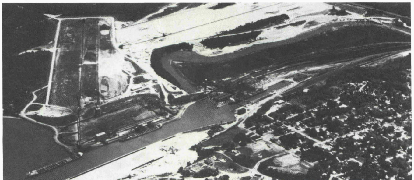
Fig. 12: The overall facilities, with the master plan nearly completed. It includes the second coal yard and dumper. The ore yard expansion and the second 10,000 t/h ore yard with its own railroad loadout station
