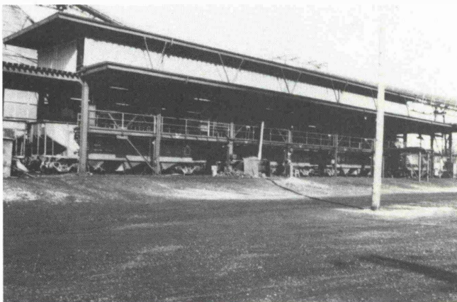
Fig. 2: Highest capacity bottom dumping installation. Silhouettes shakeouts and gates, so that a single operator, located at a distance, operates the 6 shakeouts, the train locomotive and the coal stockpiling
