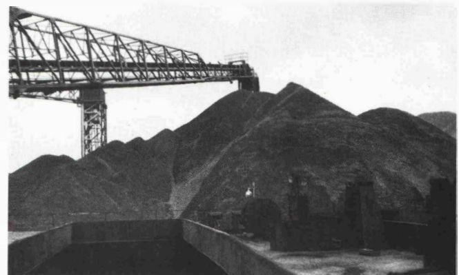
Fig. 15: View of the material discharged (crushed limestone) by MV "AGAWA CANYON" during her first unloading at Ontario Stone Dock, Cleveland, Ohio, USA
