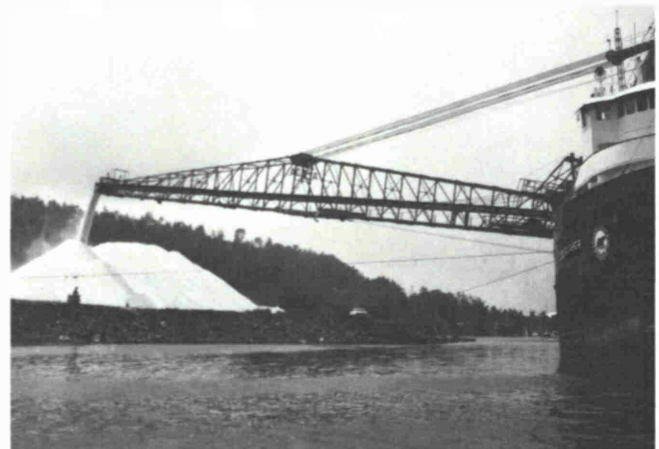
Fig. 1: Belt conveyor self-unloader with 250 ft deck boom discharging salt onto shore stockpile while moored 100 ft off an unimproved shoreline where there are no dock or shoreside handling facilities of any nature available. (Photograph courtesy of Jones, Bardelmeier & Co. Ltd.)
