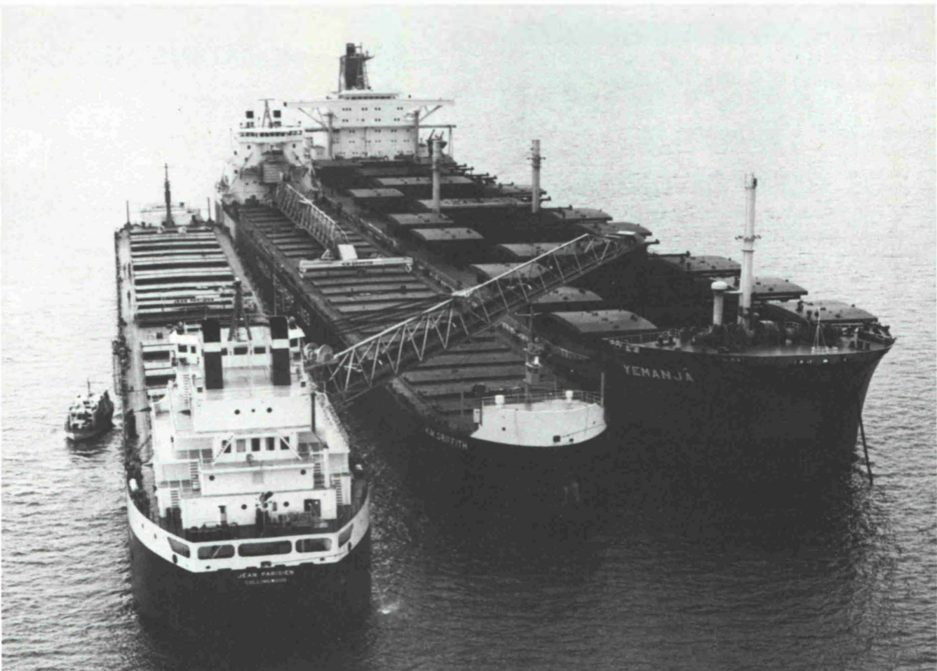
Fig. 3: Canada Steamship Lines' lake self-unloader Jean Parisien discharges 25,000 tons of coal loaded at a Lake Erie Port over the deck of her sister ship H. M. Griffith which just completed discharge, at Seven Islands directly into the 165,000 DWT ocean bulk carrier Yemanja which delivered the cargo to a steel mill in Japan. (Photograph courtesy of Canada Steamship Lines)
